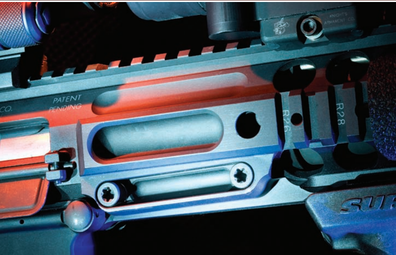
The heart of LMT's user-replaceable barrel is this quick-change interface. Two Torx screws are all that hold the barrel, yet it headspaces precisely and is locked in place. With the larger platform .308 receiver, you could switch barrels to a 7-08 or other .308-based cartridge.
