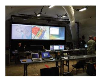
Designed to fit into a large Deployable Rapid Assembly Shelter (DRASH), the DC2E Large Screen Display system features three DLP projectors that project on to three separate large, diagonal viewing areas. Its unique configuration allows it to be set up nearly 5 feet above the floor allowing for ease of viewing from the back of the TOC. Regardless of its size, the Large Screen Display system packs down tightly into four lightweight cases.
